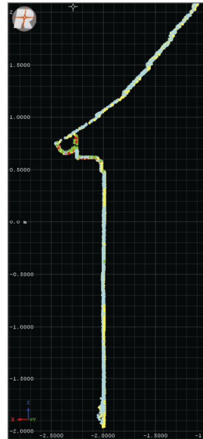
Detail of the left facade before & after the boresight alignment
